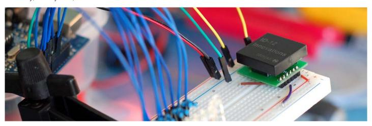
A few weeks ago we showed you how to <u>control your arduino over serial</u>. Well this week are going to do the same thing. Only this time instead of using the serial monitor to send the commands, we will be using the Innovations ID line RFID reader.
