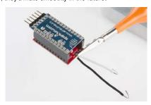
You can see a couple of points: the pin headers on the MiniGen have been soldered in with the long pins on the opposite side from the components, and the receptacles are on the component side of the Pro Mini.
