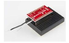
Flipping the board over, component side up, will allow you to mount it on a Pro Mini board that has female headers on its top side. I'll show you both of these cases fully assembled, so you can see the implications of each.
