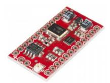
The MiniGen was designed to be used either as a stand-alone board or as a shield that can be placed on top of an Arduino Pro Mini. It's capable of generating sine, square, or triangle waves at up to 3MHz, and approximately 1Vp-p. The output is at a DC offset of Vcc/2. Neither the offset nor the amplitude can be varied.
