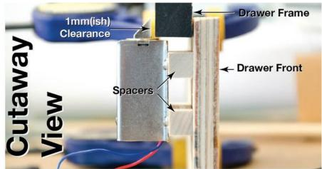
For example in the side view above, the drawer frame is 3/4" (19mm) thick. The latch has 5/16" (8mm) of clearance built in, so I need to add 1/2" (12mm) of clearance to make sure it clears the frame and can still retract fully. I used two short pieces of 1/2" square dowel.
