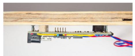
After everything is in place and tested, tack the cables in place with hot glue, cable ties, or cable staples.
