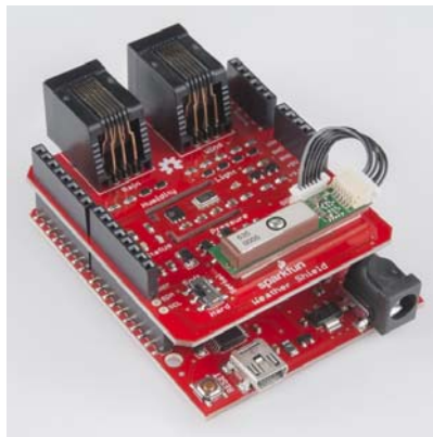
Shield on a RedBoard with optional weather meter connectors and GPS attached
