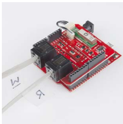
Shield on a RedBoard with optional weather meter ('W'ind and 'R'ain cables) and GPS attached
