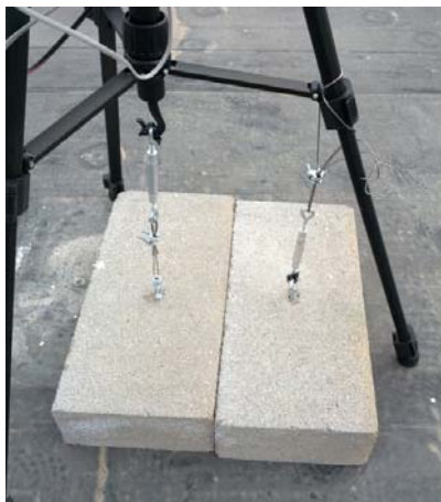
One threaded screw with inverted wing nut on the left and one eye bolt on the right
