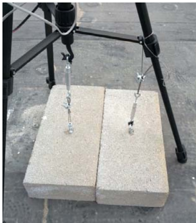
Double turn buckle with zip ties securing the connections
