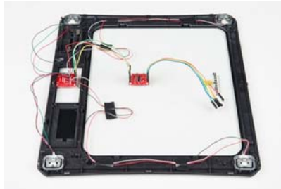
To hook up the combinator board to the HX711 match the RED, BLK, WHT, and GRN pins
