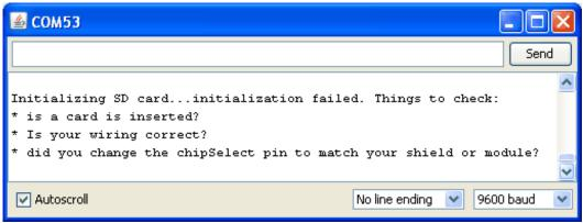
It couldn't even initialize the SD card. This can also happen if there's a soldering or wiring error or if the card is really damaged.
