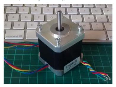
It has 200 steps per revolution, and can operate at at 60 RPM. If you don't already have the step and speed value for your motor, find out now and you will need it for the sketch.
