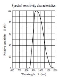
As you can see from these datasheet graphs, the peak frequency detection is at **38 KHz** and the peak LED color is **940 nm**. You can use from about 35 KHz to 41 KHz but the sensitivity will drop off so that it wont detect as well from afar. Likewise, you can use 850 to 1100 nm LEDs but they wont work as well as 900 to 1000nm so make sure to get matching LEDs! Check the datasheet for your IR LED to verify the wavelength.
