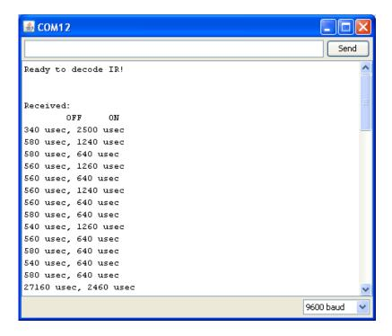
If you ignore the first OFF pulse (its just the time from when the Arduino turned on to the first IR signal received) and the last ON pulse (it the beginning of the next code) you'll find the Sony power code:
