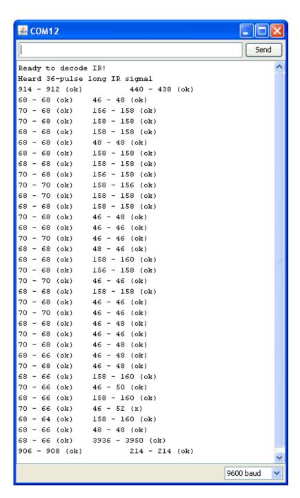
This loop, as it goes through each pulse, does a little math. It compares the absolute (abs()) difference between the code we heard and the code we're trying to match abs(oncode - ApplePlaySignal[i\*2 + 0]) and then makes sure that the error is less than FUZZINESS percent of the code length (oncode \* FUZZINESS / 100)
