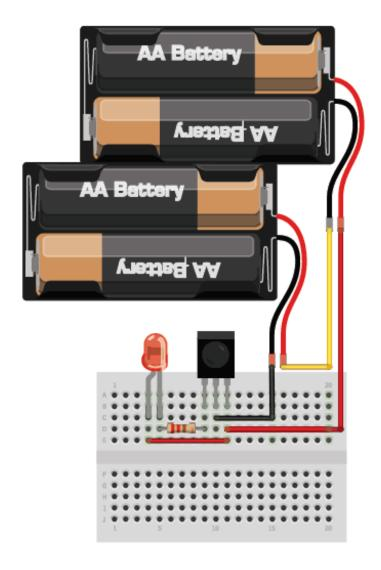
We will use 4xAA 1.5V batteries so that the voltage powering the sensor is about 6V. 2 batteries (3V) is too little. You can also get 5V from a microcontroller like an Arduino if you have one around. Ground goes to the middle pin.
