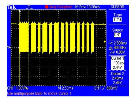
Basically we see pulses or IR signal. the yellow 'blocks' are when the IR LED is transmitting and when there is only a line, the IR LED is off. (Note that the voltage being at 3VDC is just because of the way I hooked up the sensor, if I had swapped the pullup for a pulldown it would be at ground.)
