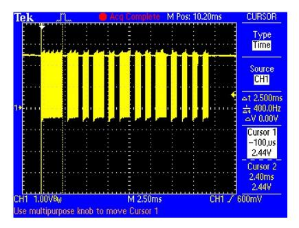
The first pulse is 2.5ms. We can use the cursors to measure the remaining pulses. I'll spare you the 12 images and let you know that the pulses are:
