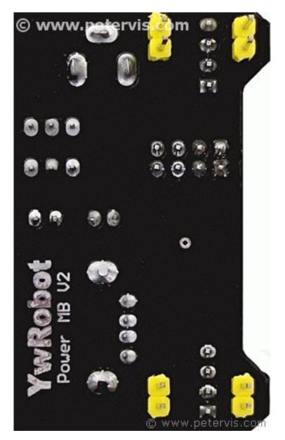
The PCB manufacturing is of good standard, and the markings indicate the model MB V2, known as MB102. This is obviously a double-sided board that is machine assembled to a good quality standard. There are two sets of mounting header pins, and the ones on the front are if you want to use the holes on the outermost edge of the breadboard thereby using a least number of tie points.
