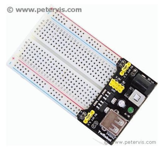
This is a plug-in power supply and the headers below the board simply plug-in to the breadboard.
