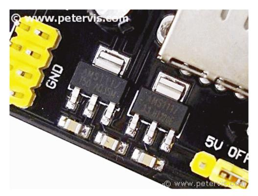
The AMS1117 is a voltage regulator manufactured by *Advanced Monolithic Systems*. There are two regulators where one regulator establishes a 3.3 V rail, whilst another establishes the 5 V rail. These are a good make of components found in a SOT-223 package. Their documentation states that this series can provide a maximum output current of 1 A, and the absolute maximum input voltage rating is 15 V.
