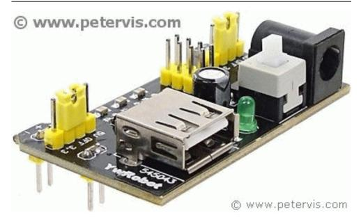
There is a green LED to indicate the presence of power, and an ON / OFF latching switch to control the power to the board. On this particular model and version, the centre pin of the barrel socket is positive; however, please
