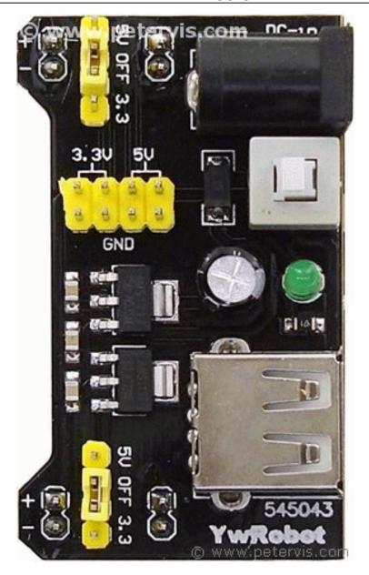
The MB102 is a *breadboard power supply module* manufactured by the YwRobot Corporation in China. This module has the marking 545043 and MB V2 on the *printed circuit board* (PCB). It provides dual 5 V and 3.3 V power rails, and has a multi-purpose female USB socket.
