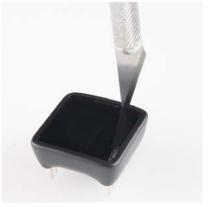
Then pry up the cover by tilting the opener towards the outside of the MicroView.
