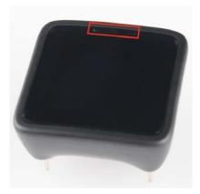
Insert your opener somewhere between that notch and the bottom of the cover. You should be able to push it in about 2mm, before a beveled edge inside the enclosure gets in the way. Be gentle, but try to push in as far as you can to get more leverage.
