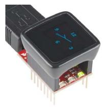
In August 2014, we (unknowingly at the time) sent out nearly 2000 MicroViews without bootloaders. Void of a bootloader, the MicroView is essentially unprogrammable – that exciting Arduino platform becomes a glorified paperweight.
