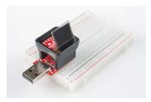
The breadboard will be useful as both a wire tie-in point and as a steadying tool.
