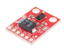
The APDS-9960 RGB and Gesture Sensor board breaks out the pins on the Avago APDS-9960 so you can easily use it in a variety of projects. The APDS-9960 uses the I<sup>2</sup>C interface for communications.
