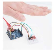
Gestures will appear on the serial monitor, which indicate the direction of the swipe.
