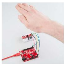
Move your hand around above the sensor, and you should see Z (height above the sensor) and X (position side to side) appear in the serial terminal.
