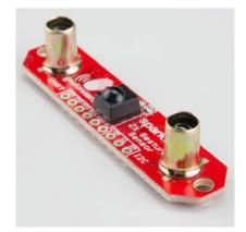
They are held on with Super Glue. You can remove them, but it might require a bit of acetone. If you plan to mount the ZX Sensors in your own housing, make sure IR light can't travel directly from the sides of the LEDs to the receiver (i.e. you will want to make your own IR shields).
