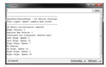
NOTE: The "Speed" of the gesture is a measure of how fast the gesture occurred. Note that the *lower* the number, the *faster* the gesture occurred (e.g. 3 being very fast and 25 being very slow).
