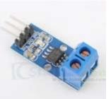
The ACS712 Current Sensors offered on the internet are designed to be easily unwith micro controllers like the Arduino.
