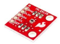
The ISL29125 breakout board, as seen above, in combination with our Arduino library makes it very easy to sense and record the light intensity of the general red, green, and blue spectra of visible light. You can use these color-intensity readings in a variety of projects: log them to find patterns or use them to creatively make control decisions.
