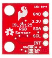
If you want to disable the on-board  $10k\Omega$  I<sup>2</sup>C pullup resistors – in case you want to use those built into your microcontroller or other external pull-ups – simply cut the two traces between the three pads on the backside of the board. If you decide you want the pull-ups later, you can always solder the pads back together.
