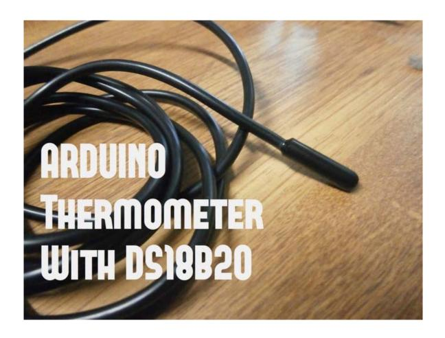
Hello, everyone! Today I'm going to show you how to use DS18B20 digital temperature sensor with Arduino, so you can measure the temperature of the air, liquids like water and the temperature of the ground.
