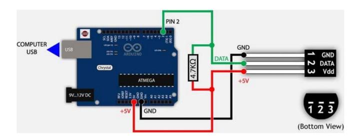
To print the data from DS18B20 on the serial monitor of the IDE you have to build the circuit by following the schematic.
