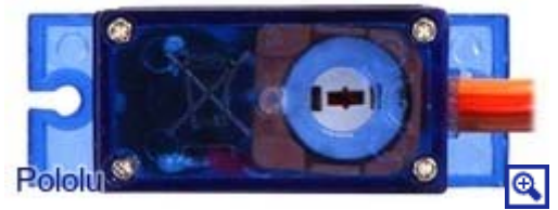
Bottom view of FEETECH FS90R micro continuous rotation servo (V1.0) showing middle-point adjustment potentiometer. FS90R V2.0 uses an SMD potentiometer.
