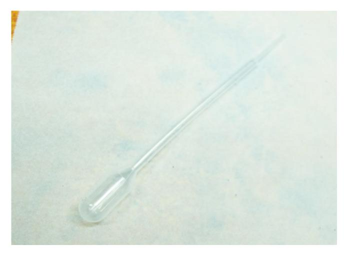
Load your pipet about half full with CA glue, and add a small amount of metal powder to the bottom of the hole. Add enough to cover the wire, but don't fill the hole at this point. Use the pipet to place a few drops of CA glue on the powder. The powder will quickly soak up the drops of glue, and you should only add enough glue to evenly saturate the powder.
