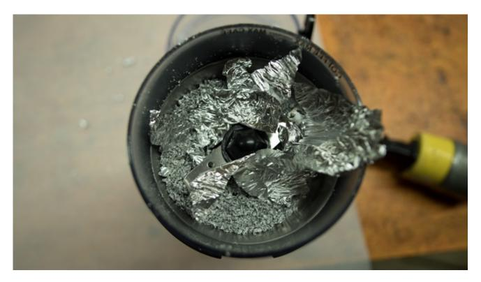
Once you get the first batch of foil ground down to about the consistency of coffee, add another batch of small foil pieces to the mix. Repeat this process until the entire one foot section of foil is in
