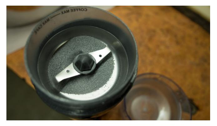
The final bit of grinding will take about 10-15 minutes. Make sure to open the coffee grinder every few minutes to expose the aluminum to air. There is a chance you could cause the fine aluminum dust to ignite if you grind for 15 minutes straight.
