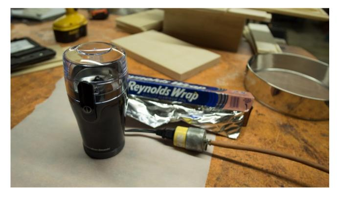
Rip off a one foot section of the aluminum foil, and fill the cup of the coffee grinder with very small pieces of aluminum foil from the one foot section. You do not need to add the entire one foot section right now, so please be careful not to overfill the grinder.
