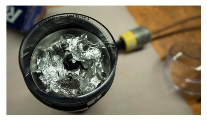
Put the lid on the grinder and start grinding the aluminum foil. Shake the grinder a bit while grinding to make sure the foil doesn't get stuck below the blades. If you feel the grinder getting hot, stop for a few minutes to let it cool down.
