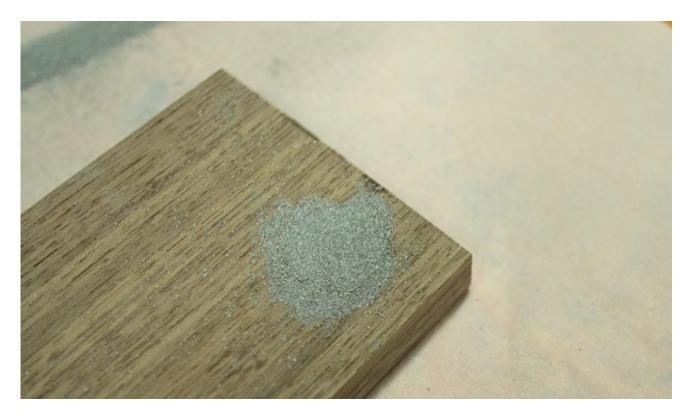
Starting from one end, start adding drops of CA glue to the powder. The CA glue will flow through the narrow spaces between the bits of metal in a process called capillary action (http://adafru.it/elj). If you ground the powder too fine, the CA glue will not be able to penetrate the powder, and it will sit on top of the powder. If this happens, you may need to grind a new batch of powder. Do not oversaturate the powder.
