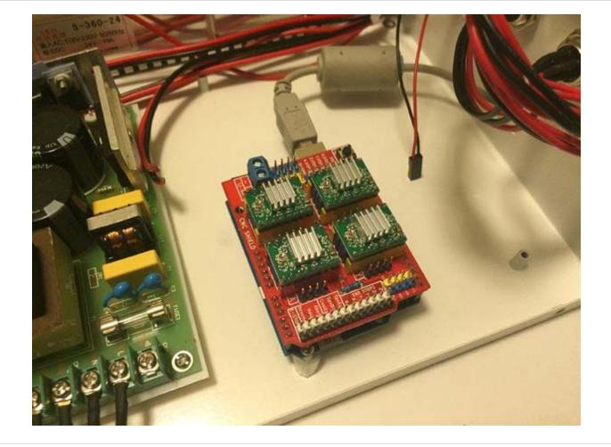
The CNC Shield has spots for 4 driver chips. It accepts the A4988 or the DRV8825, the later being more powerful and able to accept up to 36volts and 1/32 microstepping.
