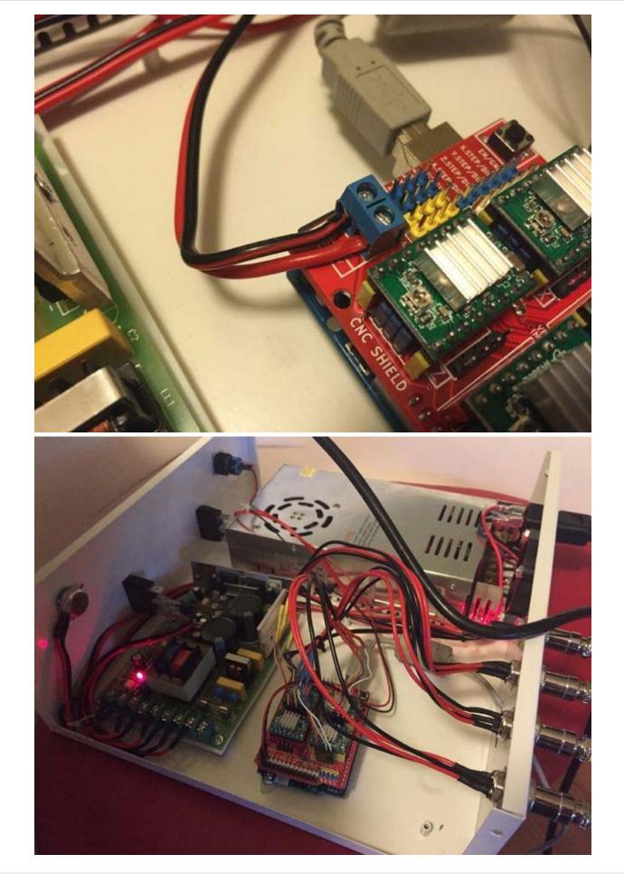
For my conversion, I have a dedicated USB cable that I put into the Arduino and it just simple comes out of the control box, I didn't bother positioning board so I can unplug it. This USB plug not only connects your computer to the Arduino, but it also powers it.
