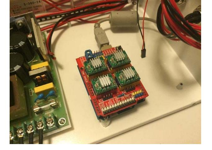
The Arduino needs to be flashed with the most current version of GRBL. What does GRBL stand for? No idea, jury's still out.
