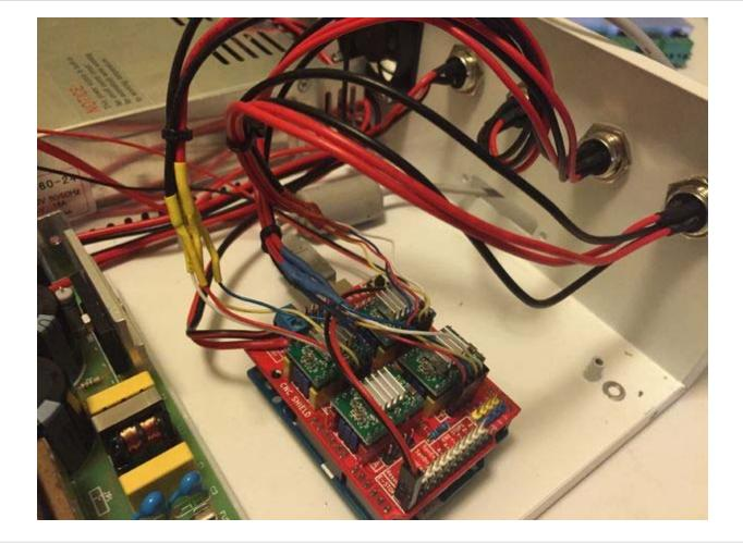
Ok...so you've removed the XYZ cables from the old driver board, the Arduino and stuff is mounted...now you need to interface the old with the new.
