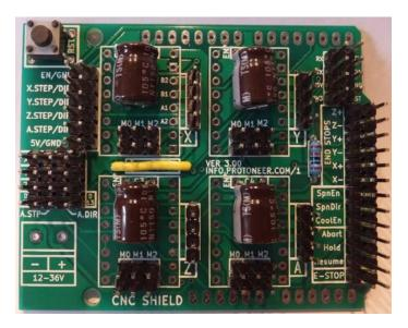
5. Before soldering the stepper driver headers in place it might be easier to solder the Arduino headers in place. I usually do it by inserting the headers into an Arduino board and then by placing the shield on top of them before I soldering them in place. This ensures that the headers are always aligned and straight.
