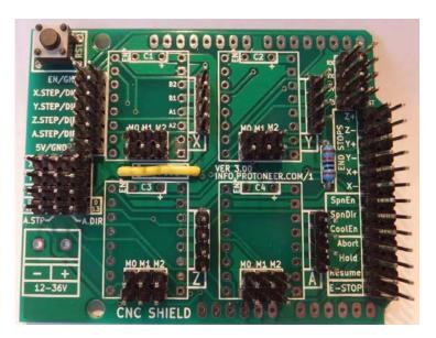
4. Because of the height of the capacitors needed, we decided to mount them horizontally utilizing all the space under the stepper drives. This also leaves a bigger
