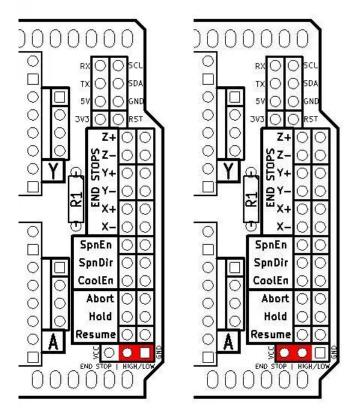
End-stop switches are standard "always open" switches. An End-stop gets activated when the end-stop pin connects to ground(When setup with default GRBL settings).
