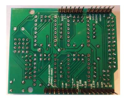
6. Last bits are to Solder the Stepper driver headers in place. I use the same principle as with the Arduino Board to align the Stepper Driver headers.
