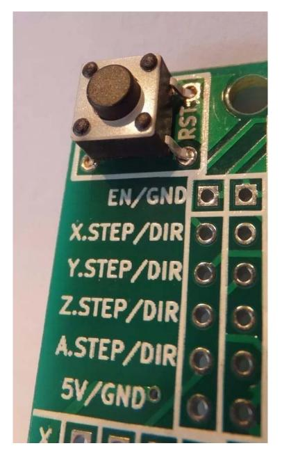
3. Majority of the assembly work is soldering the provided header pins in place. For me the easiest way is to start with pins on one side and work to the other side. By doing this the board will lean-to one side forcing the next pins you are working on to be inserted all the way into the board (Ready to be soldered in place).
