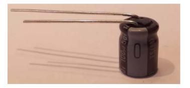
B. Then solder them in place making sure that positive lead is on the side with the "+". Capacitors are usually marked with a "-" indicating the ground/negative lead.
