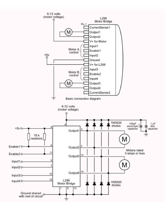
The L298 uses two different supply voltages. The voltage on pin 9 powers the chip itself and should be 5 volts. The voltage on pin 4 supplies the motors, and it can be up to 46 volts.
