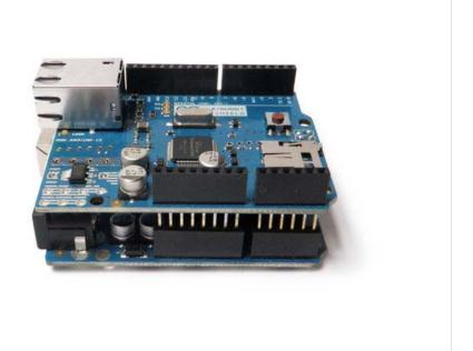
The Ethernet Shield is based upon the W51000 chip, which has an internal 16K buffer. It has a connection speed of up to 10/100Mb. This is not the fastest connection around, but is also nothing to turn your nose up at.
