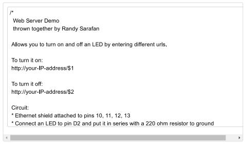
To make this work connect the positive lead an LED to pin D2, and the negative lead in series with a 220 ohm resistor to ground.
