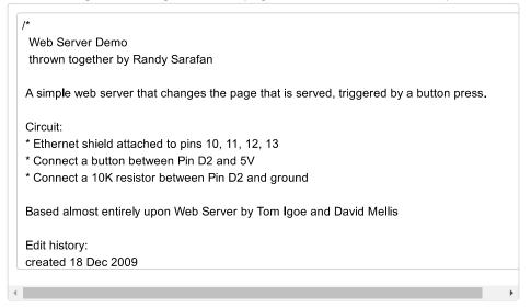
To make this example code work, simply attach a button between pin D2 and 5V, a 10K resistor between pin D2 and ground, and then load the IP address of your Arduino into your web browser. The page should load with a black background. Press and hold the button, and then refresh the browser page. The site should now load with a white background.
