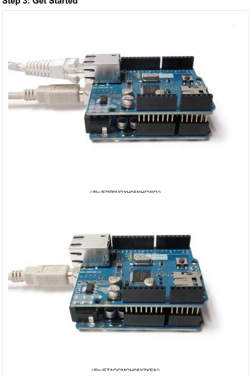
Plug the Arduino into your computer's USB port, and the Ethernet shield into your router (or direct internet connection).
