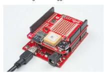
The shield is based around a GP3906-TLP GPS Module - a 66-channel GPS receiver featuring a MediaTek MT3339 architecture and an up to 10Hz update rate. The GPS module will stream constant position updates over a simple serial UART, which you can then log to a µSD card and/or use for other position or time-tracking purposes
