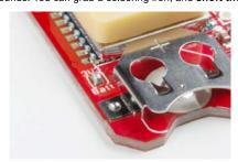
If you don't have a 12mm battery, shorting the 3V3/Batt jumper will at least keep your GPS module functional.
