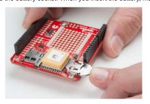
If you don't have a battery handy, there are a few workarounds. You can grab a soldering iron, and short the 3V3-Batt jumper, next to the battery socket.
