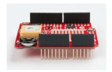
If your application requires use of the **6-pin**, **2x3 SPI header**, you may also want to solder female headers to those pins (make sure they're pointing down, and slot easily into your Arduino's male SPI pins).
