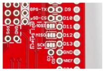
Looking closely, you'll see traces cut on all three SPI lines between the middle pad and D11, D12, and D13. That disconnects the µSD lines from those pins – leaving them connected to the SPI header.
