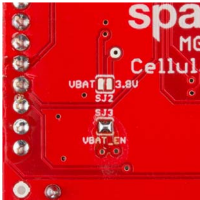
Jumper configuration for battery power. Cut SJ2, and short SJ3 (then clean it up better than we did).
