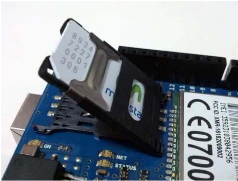
Push the SIM to the board and slide the metal bracket towards the edge of the shield to lock it in place.
