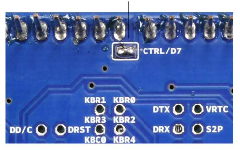
Several of the modem pins are exposed on the underside of the board. These provide access to the modem for features like speaker output and microphone input. See the datasheet for complete information.
