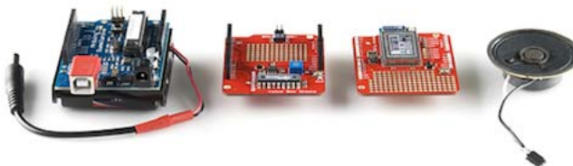
Project components - the Arduino main board with 4 AA battery pack, VoiceBox shield, WiFly shield, and speaker.
