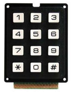
**Keypad** is a library for using *matrix* style keypads with the Arduino. As of version 3.0 it now supports mulitple keypresses.
