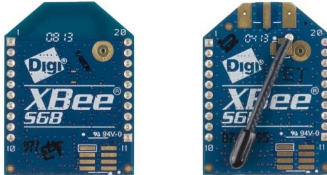
XBee WiFi modules with PCB antenna (left) and whip antenna (right). No external antenna needed!
